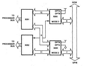
Figure 2. Talker/Listener/Controller Configuration
